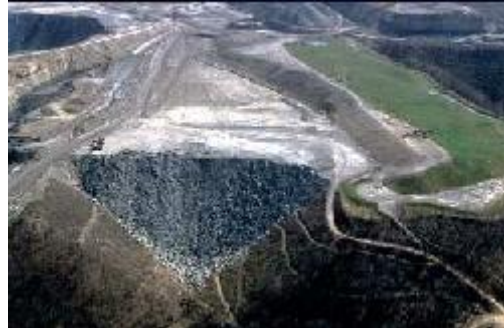
Mountaintop removal mining converts Appalachian forests into grasslands, and fills adjacent streams and valleys with mining waste. (Photo courtesy of U.S. News & World Report.)
